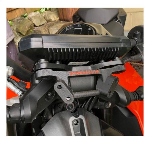
Step 3: Place the carbon screen onto the bracket and screw in the 4 M6 Bolts
