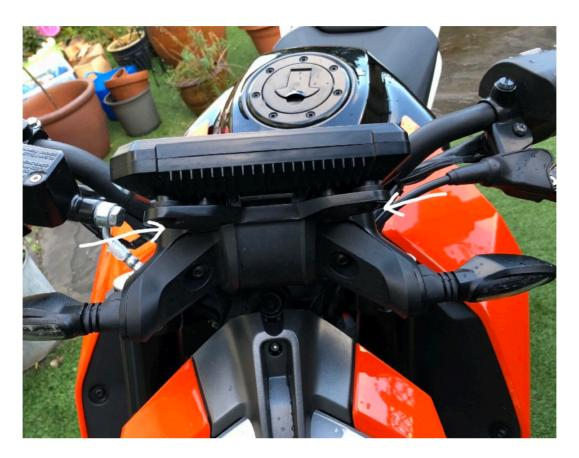
Step 2: Insert the two m5 bolts into the two holes on the bracket and screw into the back of the TFT Display
