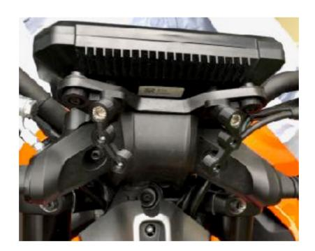
Step 6: Dry fit the Carbon screen to the front, adjust the bracket angles where needed then fully tighten them.
