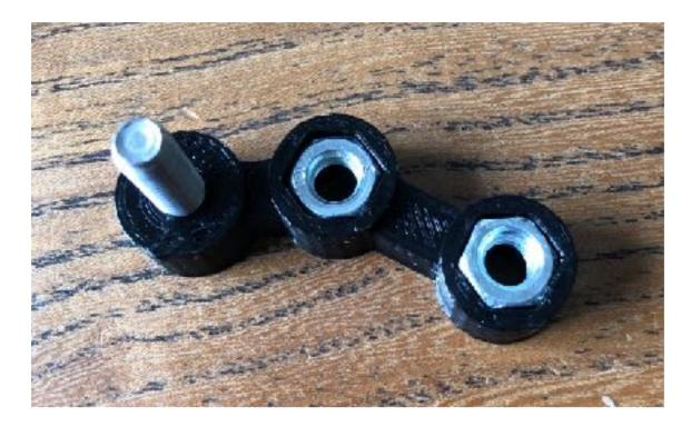
Step 2: Screw on the matching TFT brackets, with the nut hole corner pointing down towards the two nut holes. The screen brackets so end up roughly like they are in the picture below. The angle can always be tweaked once on the bike, as long as the are on the correct screen bracket.
